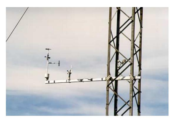
Fig. 3. Anemometers and thermometer at 10.3 - 10.8 m above the ground at Sómastaðagerði. Photo: Flosi Hrafn Sigurðsson, 1999.
